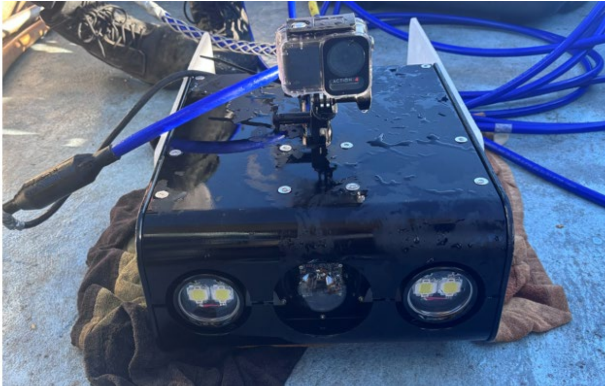
Figure 7: Technautics towed video system used for the ground-truth survey
