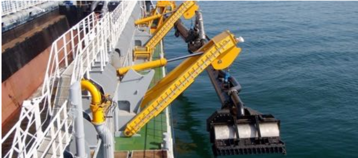
Figure 8.2 Example TSHD drag head (image source https://products.damen.com )
