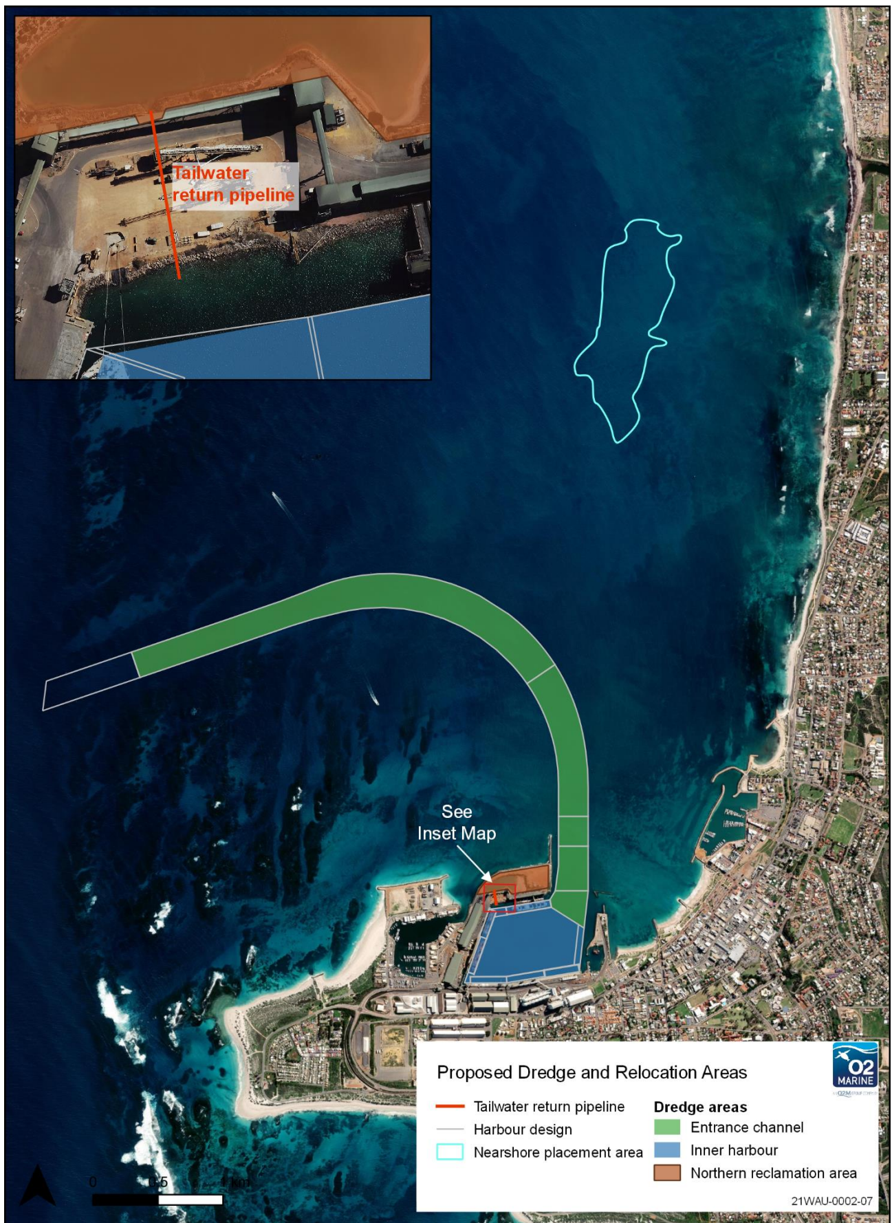
Figure 1-1 Proposed dredging and relocation footprints and associated development envelope
