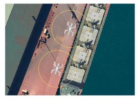
**Note**: The use of different sized outrigger arrangements will result in different localised vertical loads to those referred to in Appendix B. To seek approval for alternative load arrangements, which fall outside the conditions of the berth load capacity plans provided in Appendix B, contact the MWPA Engineering Department.
