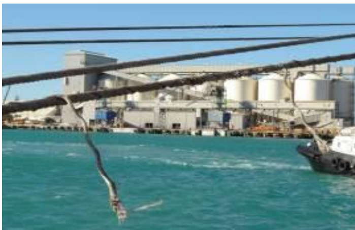
Photo 3 shows a frayed mooring line.
