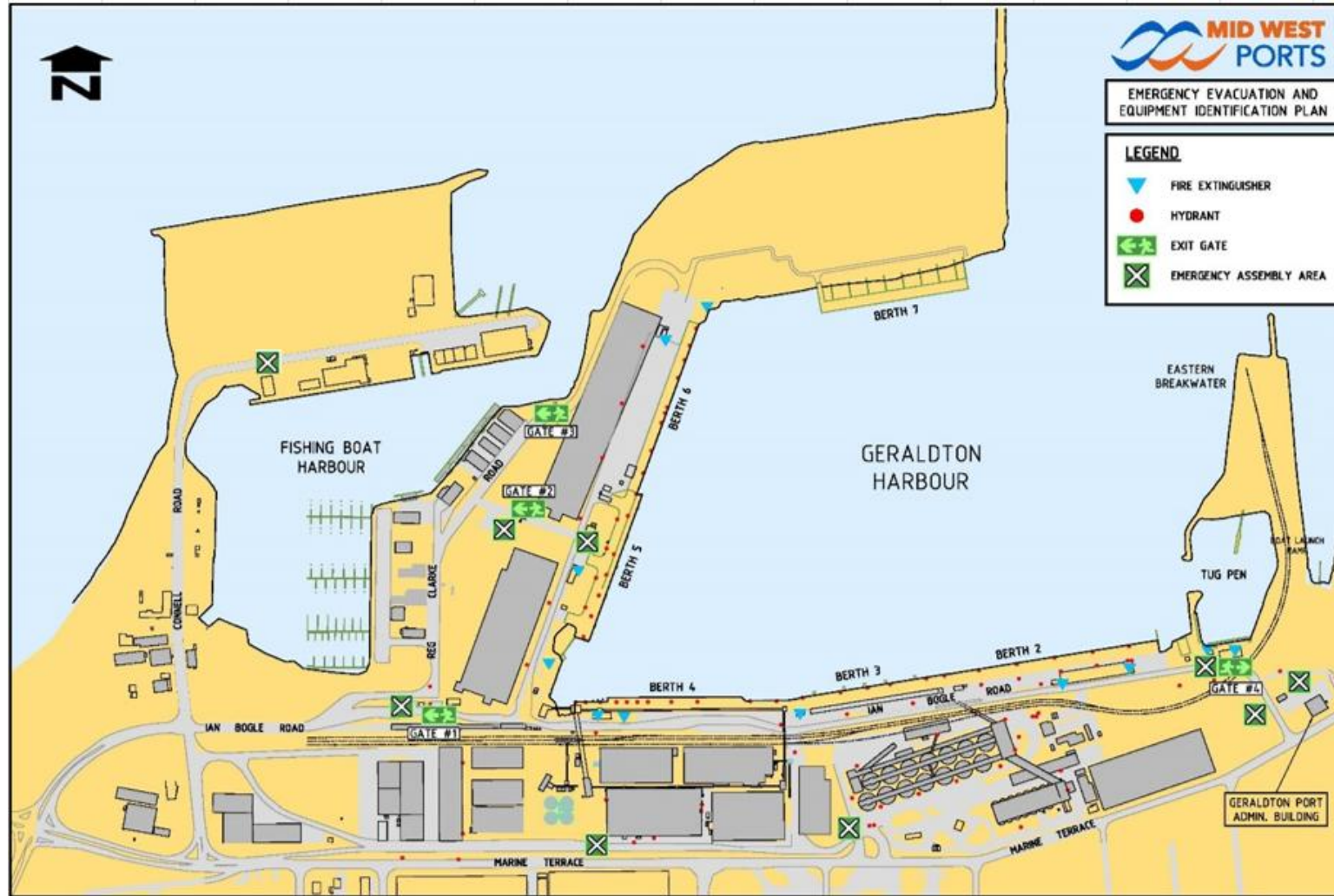
Figure 1 – MWP Emergency Equipment and Evacuation / Assembly Areas
