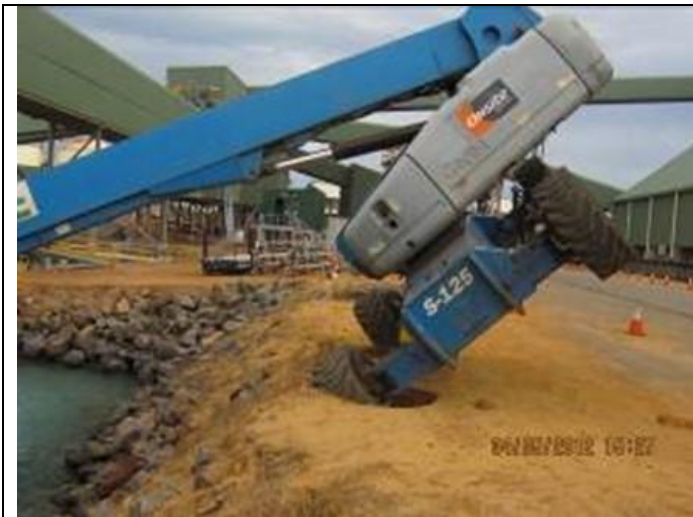
Photo 1 shows an incident where a Mobile Elevated Work Platform (MEWP) being operated close to a rock wall edge tipped due to instability of the ground surface.
