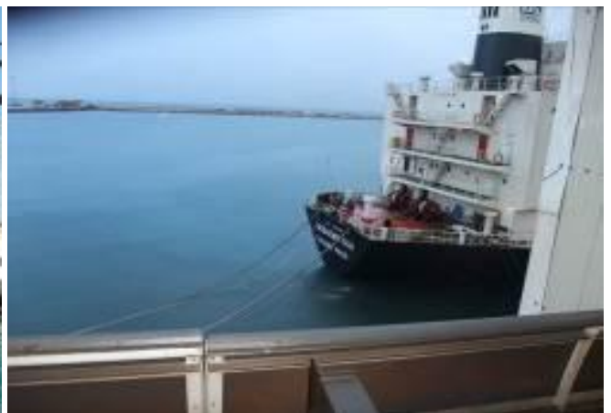
Photo 4 shows excessive slack in lines.
